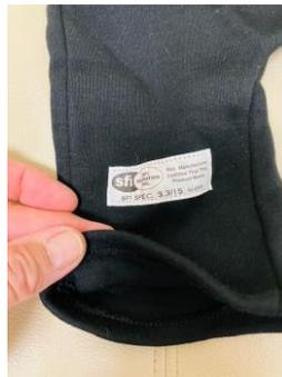
Counterfeit level 15 label on single layer Speedsy glove
