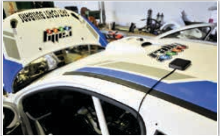
Stick-on Antenna is mounted on the ROOF of the vehicle, preferably within easy cable reach of the final RS unit mounting position allowing the cabling to then pass through the door seal and follow the cage bars back to the RS unit location.
